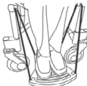
The dynamic footboard comes in one size but is able to fit most foot sizes comfortably. The height is set to length by the suspension cables and will be made to suit the user of the wheelchair. The footrest angle can also be adjusted by fixing the cable length shorter or longer, front to rear, and this can be held with a grub screw.
