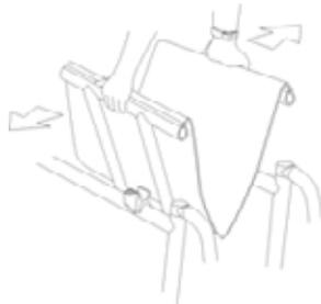
Put hands on the seat canvas with fingers pointing into the middle of seat. Push down and out, with the flat of the hand on the two sides of the seat, until the chair is completely open.
