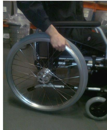
In demanding use applications, wheels are subjected to dynamic forces and increased leverage. The original build specification for 200Kg occupants and hub brakes now includes this. It is also included on high seat builds when propelling wheel diameter is increased to 26inches. A retrospective service change to this wheel in some cases may reduce damage caused by transportation tie downs.
