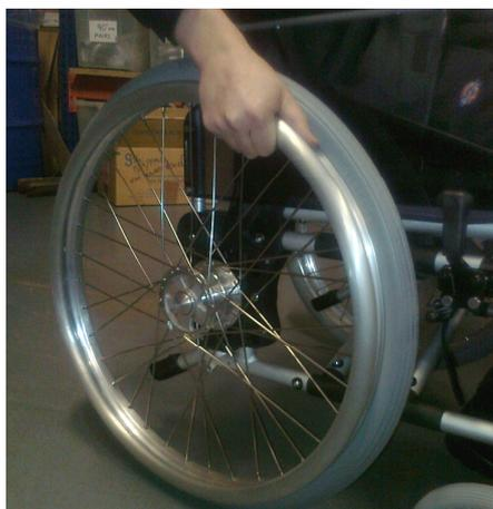
The double rim has a comfortable propelling grip feature, which for many users is a great benefit in achieving a comfortable shape for the hand when pushing.
