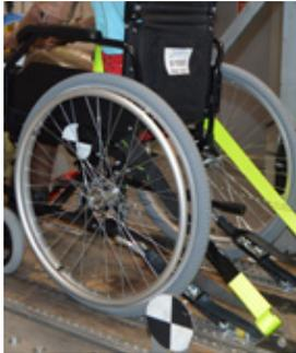
Position of the rear wheelchair tie down restraint and the tie down label on the self-propelling wheelchair.
