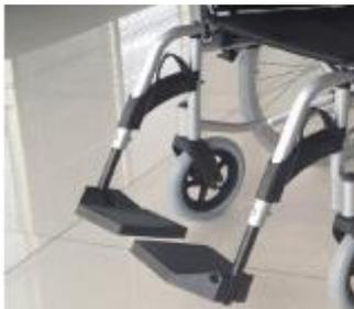
Remove the footrests. Lift the seat upholstery, as in the photo and pull up to fold the wheelchair. The back posts will also fold by operating the levers and gently pulling the posts downwards.
