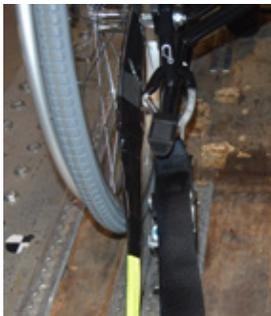
Position of the rear wheelchair tie down restraint and the tie down label on the attendant push wheelchair.
