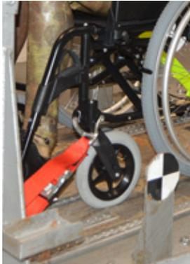
Position of the front wheelchair tie down restraint and the tie down label.
