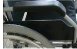
To lift the armrest, operate the lever at the front of the armrest panel and pull the armrest upwards. Simply putting the armrest downwards should relocate the armrest in position.
