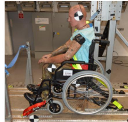
View on the left shows a self-propelling wheelchair secured with front and rear wheelchair tie down restraints. Positioning of the restraint straps is shown in more detail on the next page.
