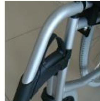
To mount the footrest, position the top spigot into the location on the front of the frame. Rotate inwards until you hear or feel them locate correctly. To remove the footrests, lift the handle and rotate footrest outward and lift upwards.
